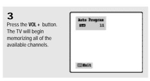
▼ The TV automatically cycles through all of the available channels and stores them in memory. This takes about one to two minutes. Press the MENU button at any time to interrupt the memorization process and return to the Channel menu.
